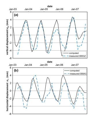
Figure 6: Matching between the ground displacement predicted by the geomechanical model and radar satellite measurements.
