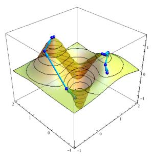
Figure 2: Gradient based optimization strategies, like the Newton method, approach fast to local optima, but the optimum reached is not guaranteed to be the global optimum, because it depends on the starting point.
