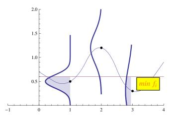
Figure 3: Graphical representation of the expected improvement for the Gaussian process example of the previous section. The thick blue curves displayed vertically represent the p.d.f. of the posterior distributions given by the Gaussian process at different sites. The purple horizontal line represents the minimum of the function obtained so far and the expected improvement at each site is represented by the blue area.
