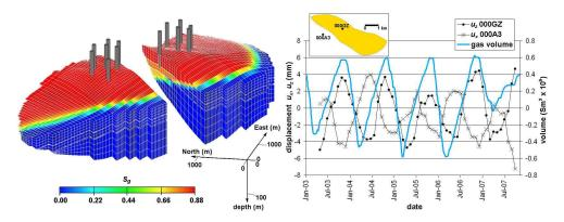
Figure 5: Panel (a): numerical model of the gas/water interaction. Panel (b): SAR measurement of the seasonal ground displacements due to injectionextraction of gas.
