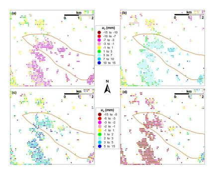
Figure 4: PSInSAR analysis of data acquired from november 2005 to april 2006 (left panels) and from april 2006 to november 2007 (right panels). The measured seasonal vertical displacements (upper panels) are of 8-10 mm and the horizontal displacements are of and 6-8 mm (lower panels). The trace of the gas reservoir is shown by the orange line.
