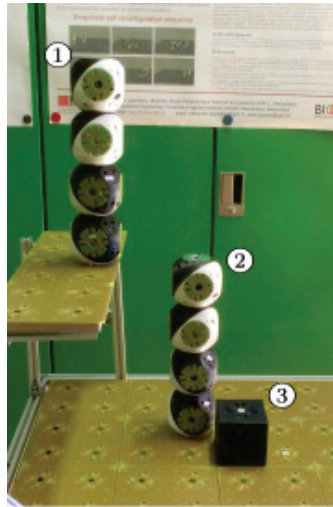
Figure 5.11 – The experimental setup: one metamodule is connected to the grid (number 1) above the second metamodule (number 2). A passive element (black cube, labeled as 3) is maintained in position using a magnet. Metamodule 2 will grab the passive element and hand it to the first metamodule.
