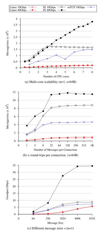
Figure 3: Multi-core scalability and high connection churn for 10GbE and 4x10GbE setups. In (a), half steps indicate hyperthreads.
