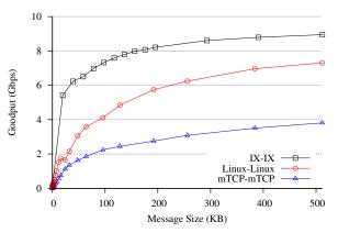
Figure 2: NetPIPE performance for varying message sizes and system software configurations.
