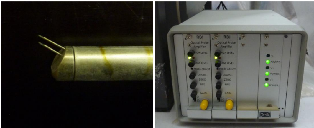
Figure 3.8. Detail of the double-fiber optic probe (left) and opto-electronic module (right), supplied by RBI instrumentation.
