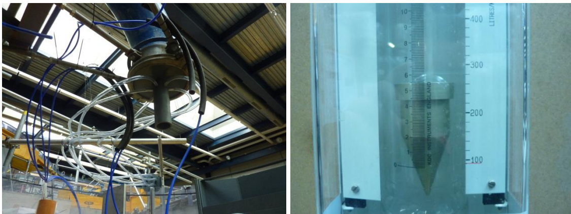
Figure 3.3. Photos of nozzle aeration devices; (left) aluminum tubes at the nozzle connected to flexible tubes; (right) air flowmeter.
