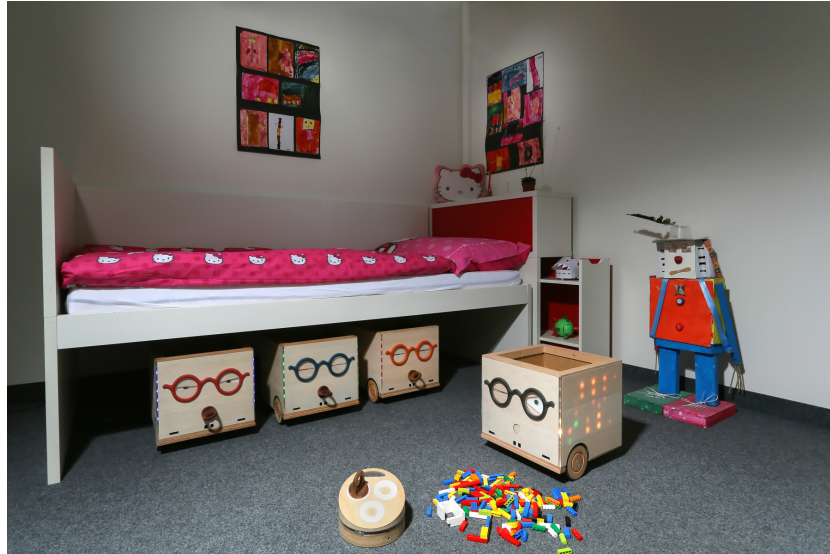
Fig. 1: A set of ranger robots in a room. Their home is under the bed, where they sleep recharging their battery. Photo: Alain Herzog.
