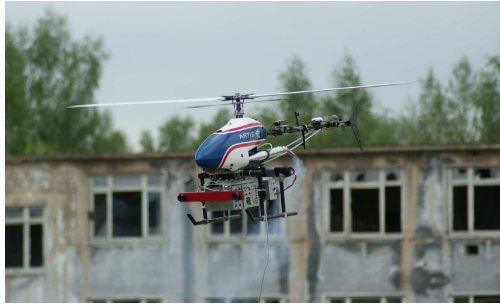
Fig. 1 Automated helicopter midiARTIS of the German Aerospace Center, maximum-take-off-weight 14 kg, rotor-diameter 1.8 m
