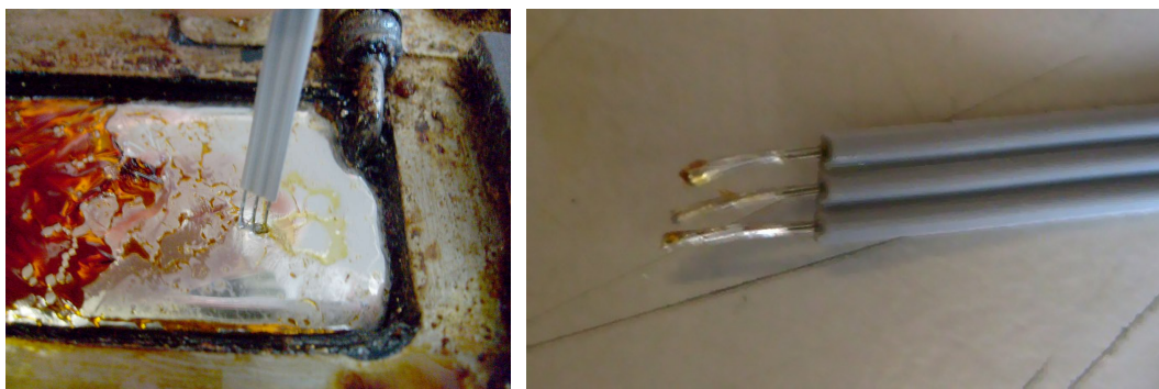
Figure 3. Tinning wire ends by dipping into molten solder (left), and resulting wires (right).
