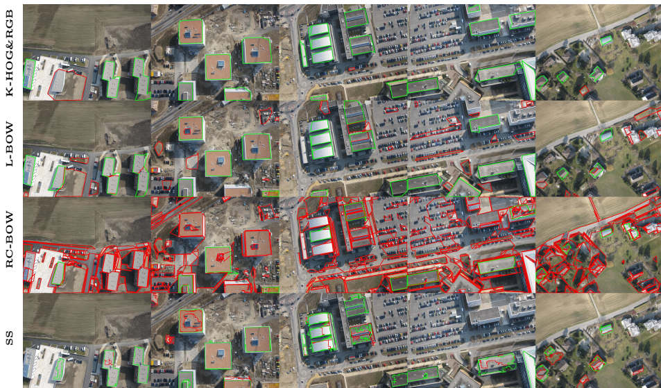
Fig. 4. Rooftop Detection. Rooftop detections obtained by our approach and the baselines are displayed at a 50% recall rate. Correct detections are shown in green and false ones in red. Our approach significantly outperforms the baselines. Unlike bag-of-words, HOG not only encodes object appearance but also its global shape which can offer a better description of the polygonally shaped rooftops in these images and likely accounts for its better performance over ratio-contour. Additionally, false detections result in missed rooftops for ratio-contour, that do not degrade the recall of our approach even when using a bag-of-words scoring function. Best viewed in color.
