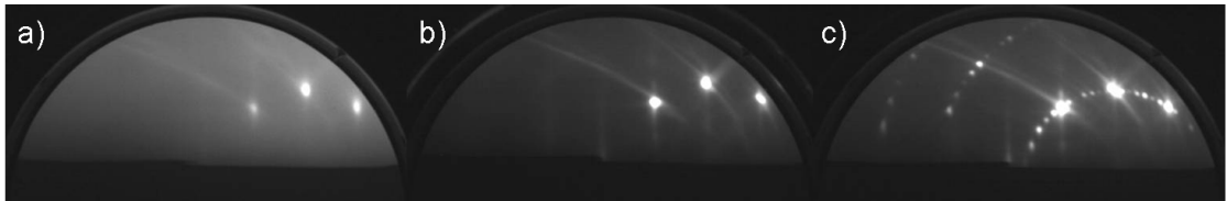
Figure 2.11: RHEED observations of the sample during a degasing (a) at 600°C, (b) 1000°C and (c) during the cooling down which allows to see the 7x7 transition.
