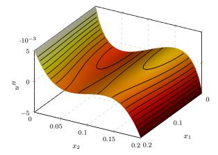
(a) FE-HMM with Dirichlet coupling,  $\delta=32\varepsilon$  and  $N_{mic}=1024.$
