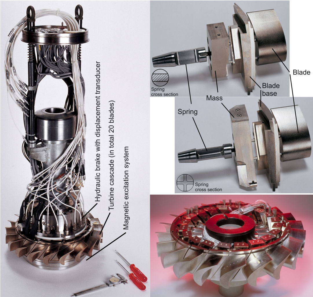
Figure 3.4: On the left: turbine cascade assembly with excitation system, measurement equipment, connector support and hydraulic brake. On the top right: one bending blade-suspension system; in the middle right: one torsion blade-suspension system; at the bottom right: turbine cascade.
