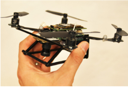
Fig. 11: Our nano quadrotor from KMeiRobotics: a 150g and 18cm sized platform equipped with an integrated Gumstix Overo board and MatrixVision VGA camera.
