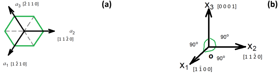
Figure 3.3: The HCP crystal. (a), crystal index of HCP in the Basal plane; (b), Cartesian coordinate definition.
