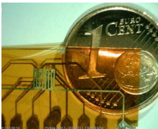
Figure 1.4: Optical picture of the sensor developed in [25]. A silver heater was printed on the bottom part of a polyimide foil and four comb electrodes on the other side of the foil to be functionalized for ammonia sensing.
