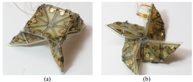
Figure 1. Examples of different shapes a Robogami can transform into (a) table (b) pinwheel (reprinted with permission from the authors) [1].
