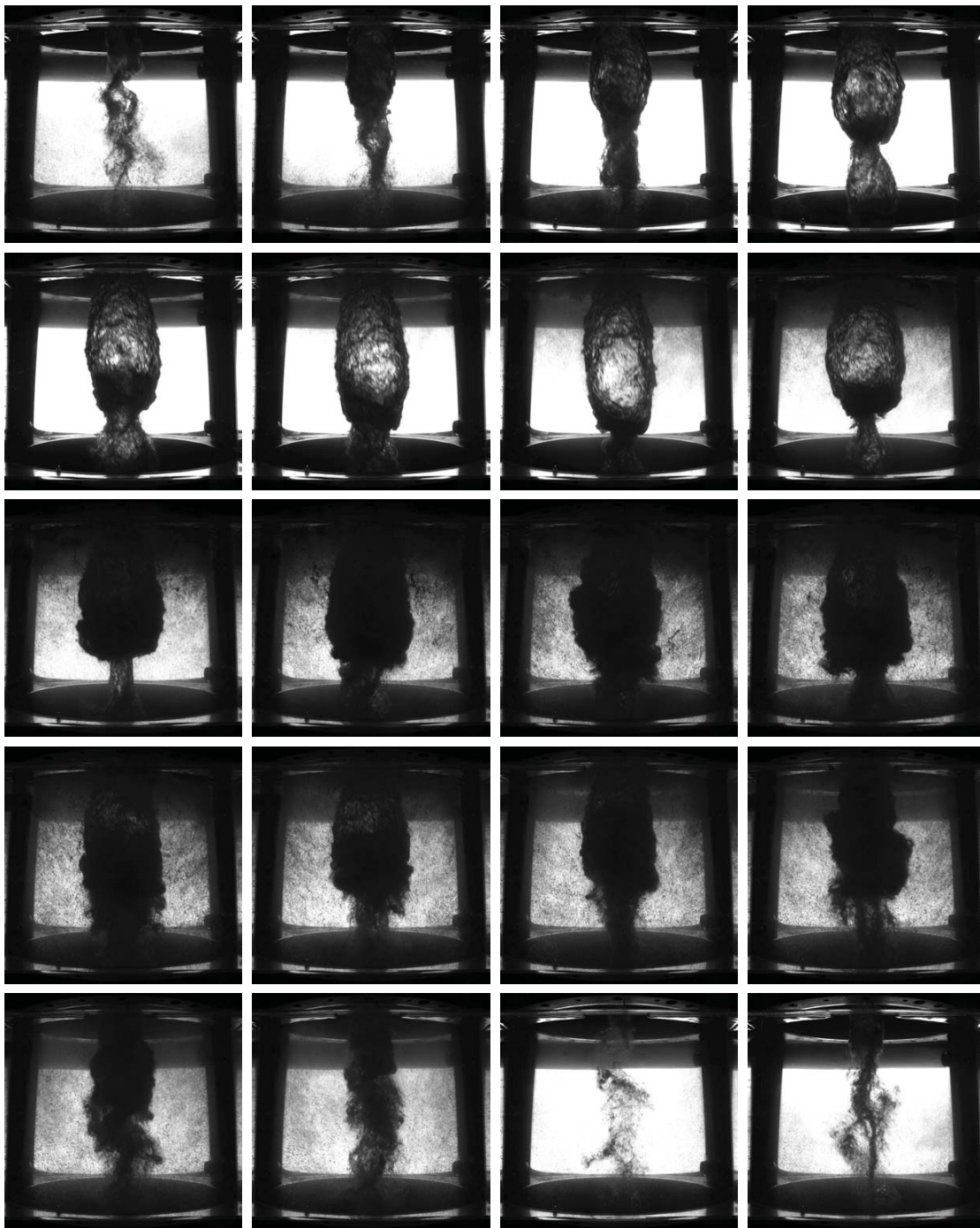
Figure A.3: High-speed visualization of the cavitating vortex rope between two pressure peaks at OP#2. The period of the oscillation is T = 0.711 s and the time increment between the photos is \Delta t = 37.4 ms.
