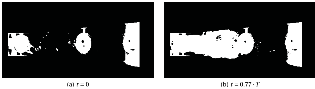
Figure 2.10: Masked binary images of two instances where the vortex rope overlaps with the pressure sensors p_4 and p_5 from Figure 2.7.
