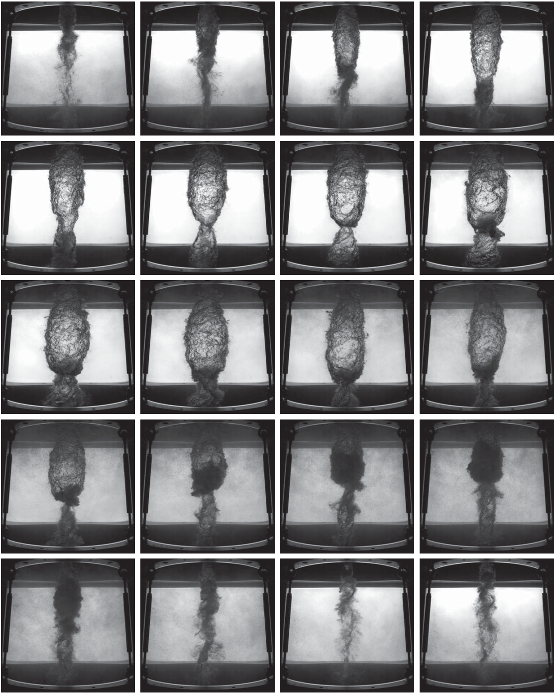
Figure 1.4: High-speed visualization of the cavitating vortex rope at OP#1.
