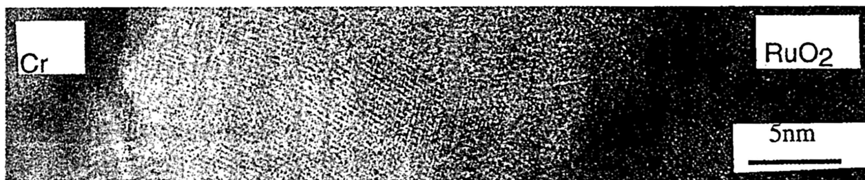
Figure 3: High resolution TEM image of the interdiffusion layer (in the middle) between the Cr and the RuO 2 .
