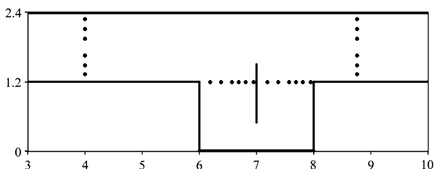
Fig. 6 Six UVP transducers distributed across a the interface section between the refuge and the channel and b the channel sections upstream and downstream of the shelter
