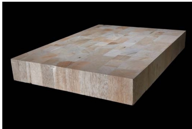
Figure 4.1: Balsa panel composed of adhesively-bonded balsa blocks (dimensions 1200 x1200 x 60mm)
