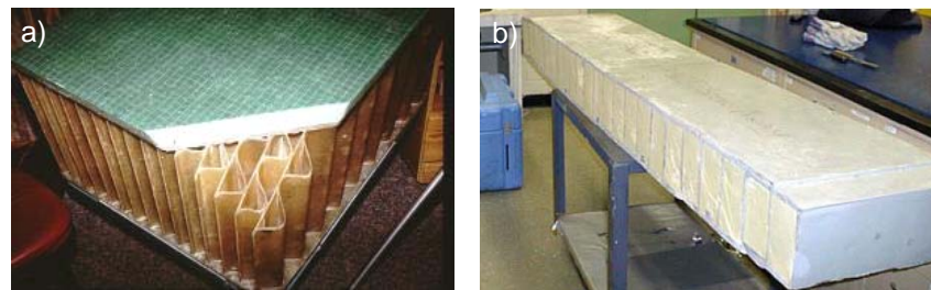
Figure 1.3: Sandwich decks with (a) honeycomb core (Kansas Structural Composites) and (b) foam core with internal GFRP webs (Hardcore Composites)
