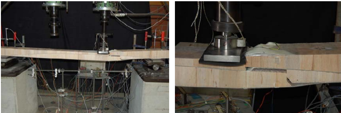
Figure B.64: Failure of beam A-G-3 (left), zoom of detailed failure mode (right)
