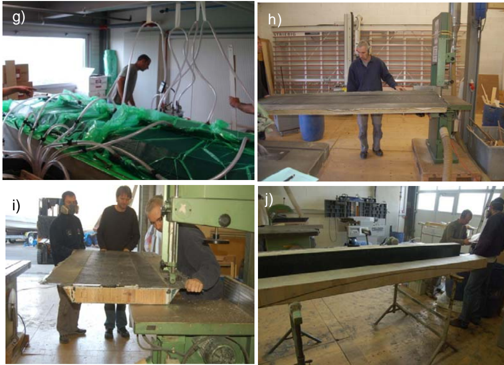
Figure B.3: (g) vacuum infusion, (h) fully infused sandwich panel (i) cutting of panels with Sesto manual saw, (j) panels cut into three beams
