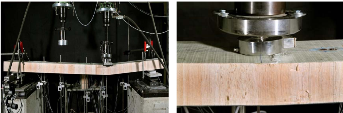
Figure B.73: Failure of beam B-L-3 (left), zoom of detailed failure mode (right)
