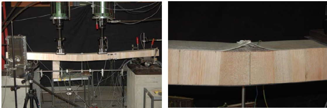
Figure B.69: Failure of beam B-H-2 (left), zoom of detailed failure mode (right)
