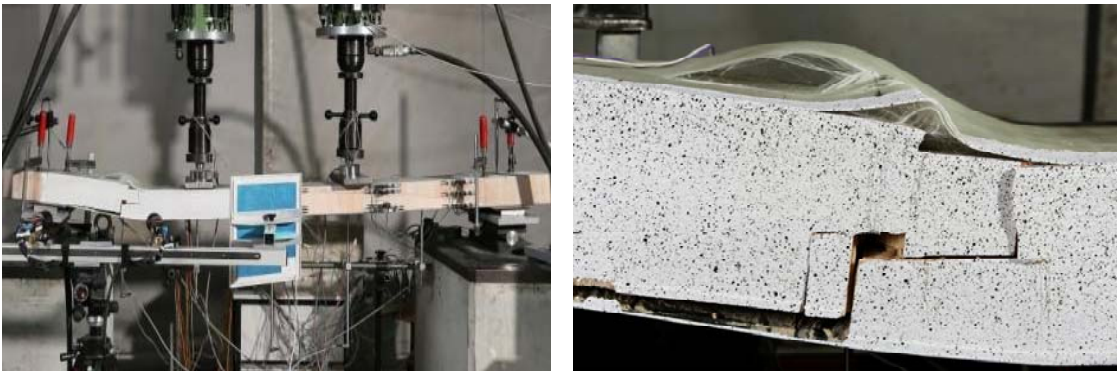
Figure B.66: Failure of beam B-H/L-2 (left), zoom of detailed failure mode (right)
