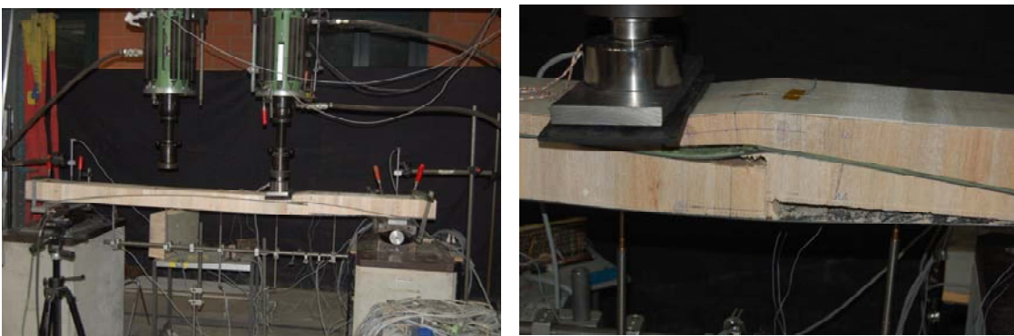
Figure B.61: Failure of beam A-C-3 (left), zoom of detailed failure mode (right)
