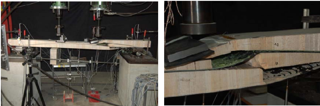
Figure B.60: Failure of beam A-C-2 (left), zoom of detailed failure mode (right)
