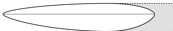
Figure 6.1: Guide vane profile. The grey area shows the region favorable for flow separation in pumping mode and the dashed lines the two horizontal tangents.
