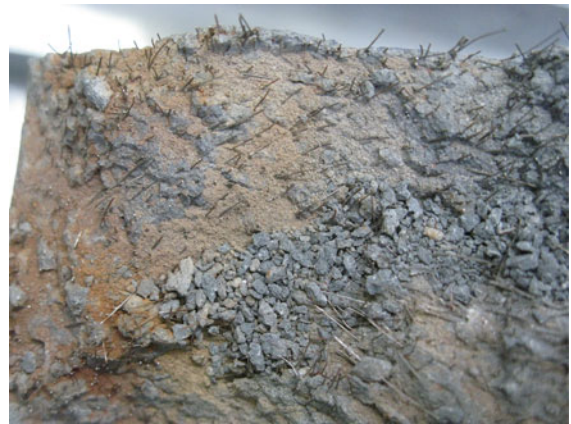
Fig. 12 Fracture surface showing matrix spalling and pulverization
