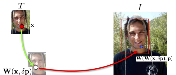
Figure 3: Updated warp in the Forward Compositional algorithm. The warp increment \mathbf{W}(\mathbf{x}, \delta\mathbf{p}) is shown as a green arrow.
