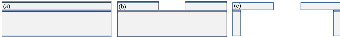
Figure 3. Fabrication steps for the extractor wafers. The SOI wafers have 50 \mu\text{m} thick device layer, 2 \mu\text{m} thick buried.
