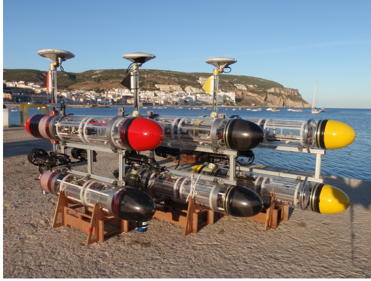
Fig. 2. The MEDUSA AMVs being readied for deployment at an experimental site.
