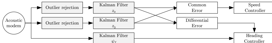
Fig. 3. Structure and data flow in the MEDUSA implementation of the formation control algorithm. Modules in grey perform the conversion of available discrete data to the continuous signals required the algorithm.
