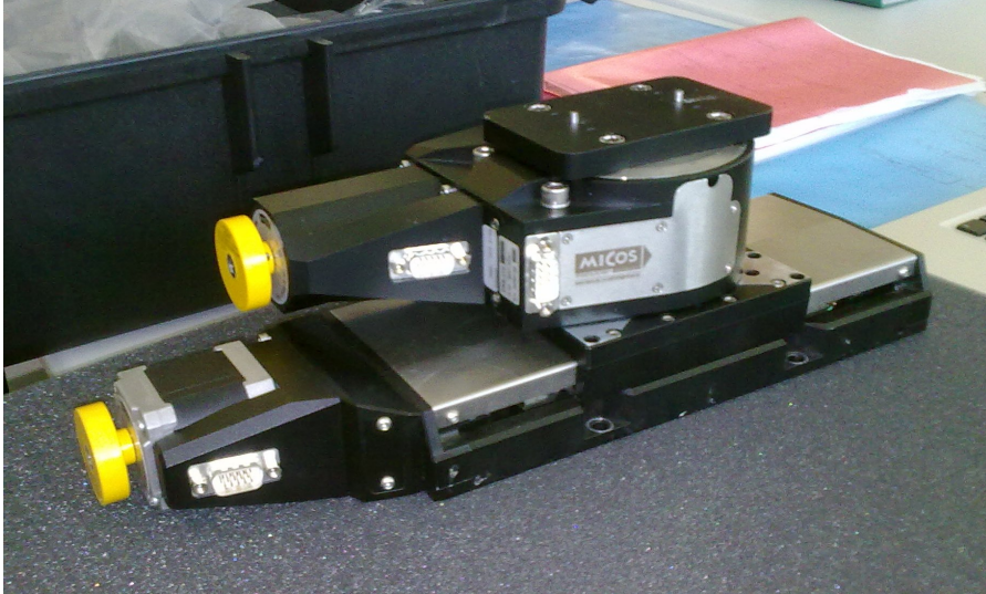
Fig. 4.4. Bottom part of the goniometer used in the UA9-H8 experiment, including the linear stage and the rotation stage of the goniometer used in the H8 experiment : movement along x (bottom) and rotation about the vertical axis (top).
