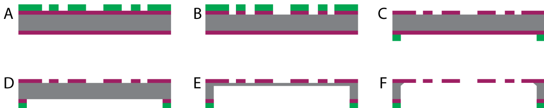
Figure 2.8: Stencil mask fabrication. A ): a photoresist mask is first made, with the designed apertures. B ): these apertures are transferred into a SiN film, via dry etching. C ): photolithography is performed on the bottom of the wafer as well, and the SiN film is also etched as before D ). E ): DRIE is used in order to create an opening below the SiN front membrane, which is finally suspended using KOH etching F ).
