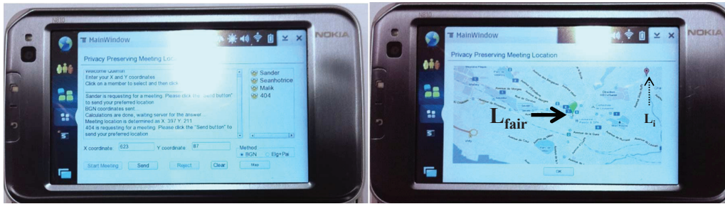
Figure 3.7: Prototype PFRVP application running on a Nokia N810 mobile device. The image on the left is the main window, where users add the desired meeting participants. The image on the right is the map that shows the fair rendez-vous location (green pin) and the user-preferred rendez-vous location (red pin).
