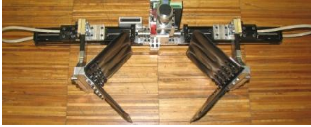
Fig. 7. Gripper of the 3DCLIMBER robot
