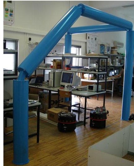
Fig. 11. Developed structure for test of the pole climbing robot.
