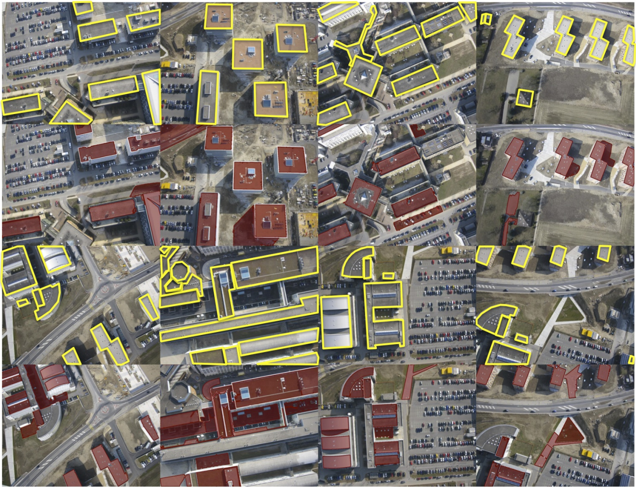
Fig. 10 Rooftop detection. Detected rooftops are highlighted in red, ground-truth rooftop annotations are shown in yellow. Our approach faithfully detects many of the relatively featureless, regularly shaped rooftops displayed in these images. False detections largely consist of other regularly shaped, constant textured regions including polygonal side-walks and courtyards.
