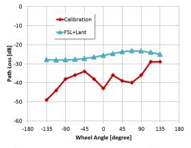
Fig. 4. Comparison between FSPL model and PL measured for the calibration setup (i). Lant are the antenna and cable losses  $\sim$ 25dB.
