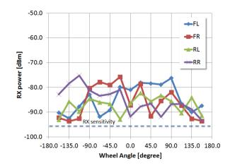
Fig. 6. Received power at 2.4GHz for the RX antenna positioned in the setup (ii).  $P_{TX}$ =2.5dBm and estimated antennas losses are 8dB.
