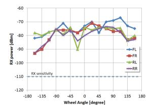
Fig. 5. Received power at 434MHz for the case of setup (i) versus wheel angle.  $P_{Tx}$ =10dBm and estimated antennas and cables losses are 25dB.
