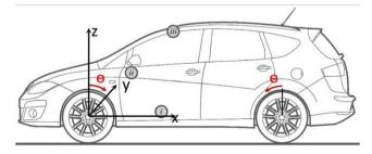
Fig. 2. Receiver position inside the car: (i)- RX Antenna in the door pocket [105, 0, 30] cm. (ii)- RX Antenna on the central console [95, 85, 70] cm, (iii)- RX Antenna on the ceiling light [95, 85, 100] cm.
