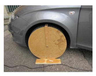
Fig. 1. Transmitter located on the wheel [0, 0, 30] cm. Origin of the coordinate system is the center of the front-left wheel
