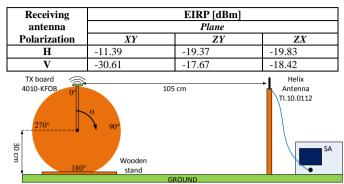
Fig. 3. Schematic representation of the calibration setup (434MHz, setup i).
