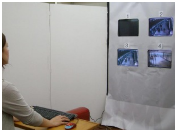
Figure 2: The setup for the Virtual Operator experiment on social attention. The subject is exposed to 4 synchronized videos. Whenever something interesting is happening on one of the screen, the user have to press the button corresponding to the screen. Every two minutes, the videos are changed; and b) an illustration of the window-based and Gaussian-smoothing-based filtering for button clicks.
