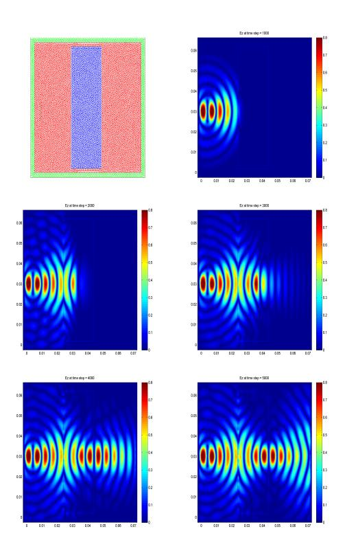
Figure 1: Example 3. The mesh and contour plots of  $|E_z|$  obtained with  $h = 2 \cdot 10^{-4}, \tau = 0.1 ps$  at 1000, 2000, 3000, 4000, and 5000 time steps.
