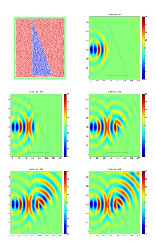
Figure 2: Example 4. The mesh and contour plots of  $E_z$  obtained with  $h = 2 \cdot 10^{-4}$ ,  $\tau = 0.1 ps$  at 1000, 2000, 3000, 4000, and 5000 time steps.
