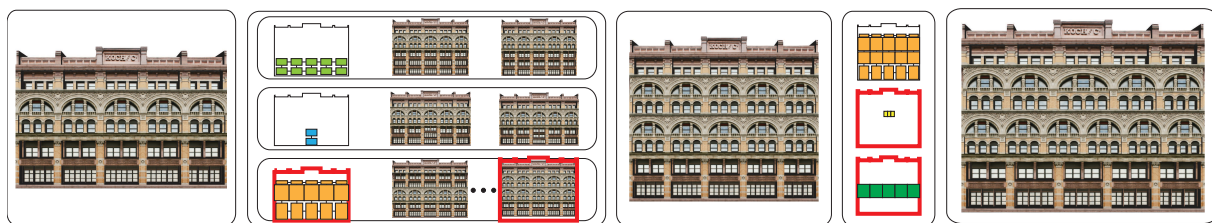
Figure 1: Structure-aware facade editing. Using the notion of generalized grids, our system encodes various symmetry, alignment, and hierarchy relations among the elements of a facade. During incremental editing, the user can specify different grids (shown as box abstractions) for which our system proposes new configurations. Editing progresses by selecting such grids and one of the proposed configurations (shown in red).
