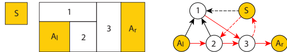
Figure 5: Connecting the source S to all the neighbors of the anchors A_l and A_r results in a conflict: the loop (S, 2, 3) suggests that S is both to the left and right of 3 . (Vertical and horizontal edges are shown in black and red respectively.)
