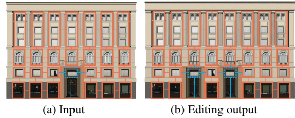
Figure 11: The door of the facade, that spans the bottom two rows, is assigned to the lower row, a phantom element (cyan) is added to the upper row.
