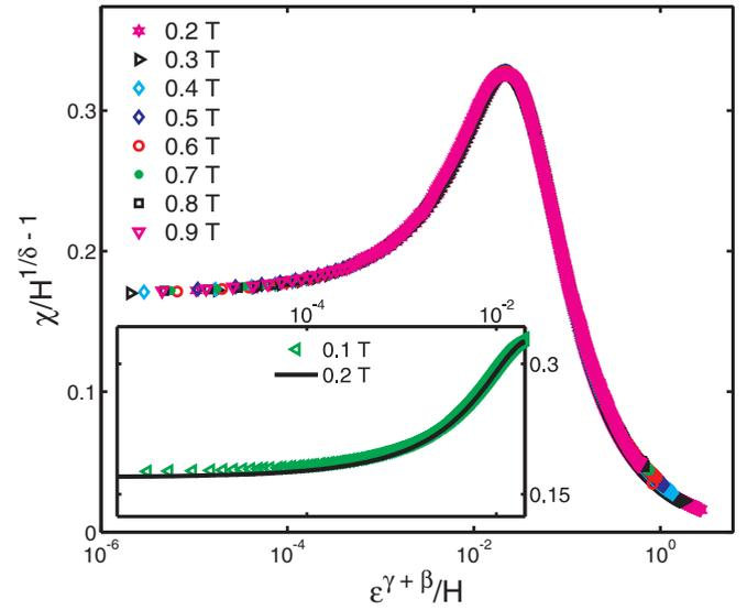
FIG. 2. (Color online) The analysis of the susceptibility measured in magnetic fields  $\mu_0 H \geq 200$  mT according to the scaling hypothesis. The parameters used are  $T_C = 58.3$  K,  $\delta = 4.9$ ,  $\beta = 0.37$ , and  $\gamma = 1.44$ . Inset: Comparison of 100- and 200-mT scans very close to  $T_C$ .
