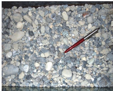
Figure 3.5: Sediments used for the mobile bed substratum.
