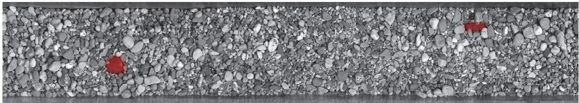
(a) Low bedload transport, at a normalized time of about t^* = 0.15 (cf. Figure 5.6f).
