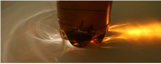
Figure 2: Reflective and refractive caustics caused by a plastic bottle filled with water, clearly distinguishable by their color.
