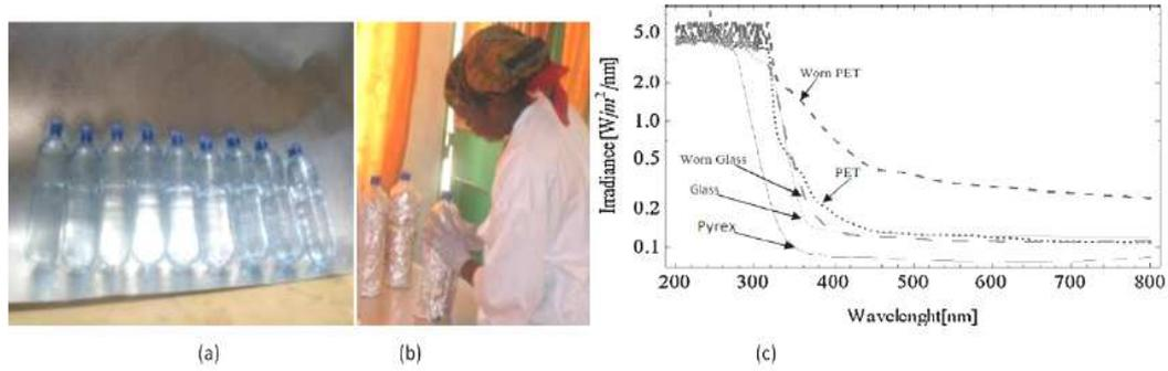
Fig. 1. (a) 9 PET bottles for the triplicate simultaneous exposure of the systems  $H_2O_2/Fe^{2+}/hv$ ,  $H_2O_2/hv$ , and  $hv$  (irradiation only). (b) Blank of each system, (c) Absorbance of different reactor materials (Pyrex, Glass, PET).
