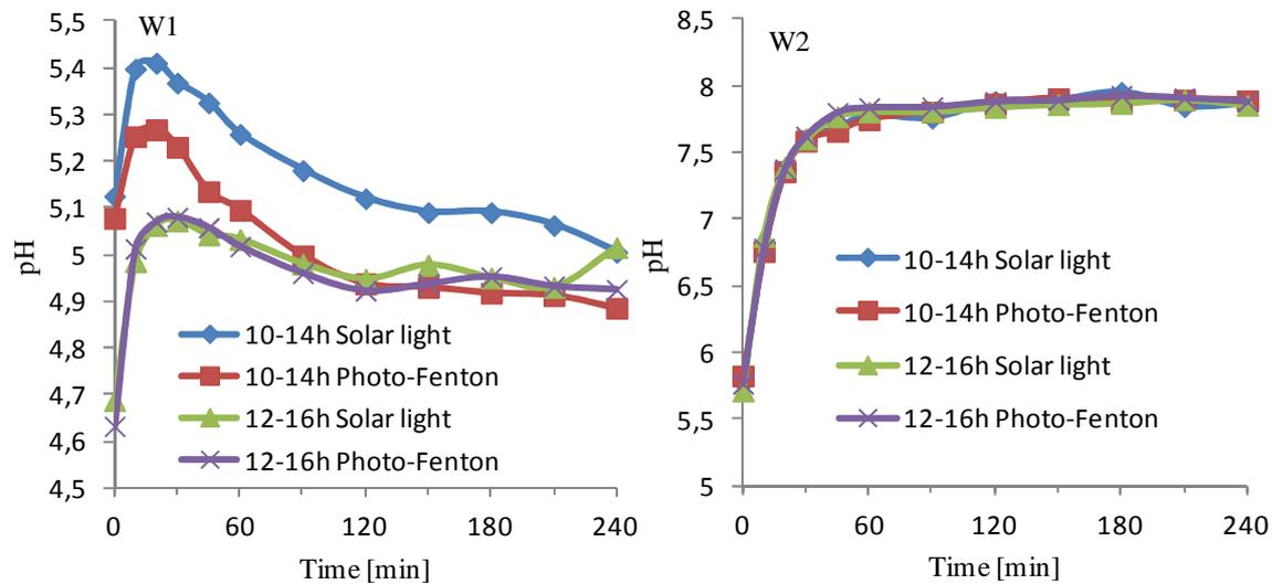
**Figure 5.1:** pH evolution during the photo-disinfection during raining season of wells 1 (Tanghin) and 2 (Nonsin) under solar light exposure and neutral photo-Fenton recorded at different day time's intervals. Bicarbonate ( $\text{HCO}_3^-$ ) concentration: in W1 ( $1.22-4.88 \pm 1$  mg/L); in W2 ( $34.16-42.7 \pm 1$  mg/L).
