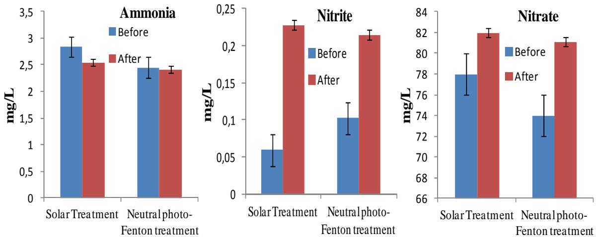
**Figure 3. 6.** Evolution of Ammonia, Nitrite and Nitrate concentration during the neutral photo-Fenton and sole solar treatment of natural well water. (notice that the difference in the initial concentration of each chemical component in the results presented here are related to the fact that new water sample was collected and used for each new experiment).
