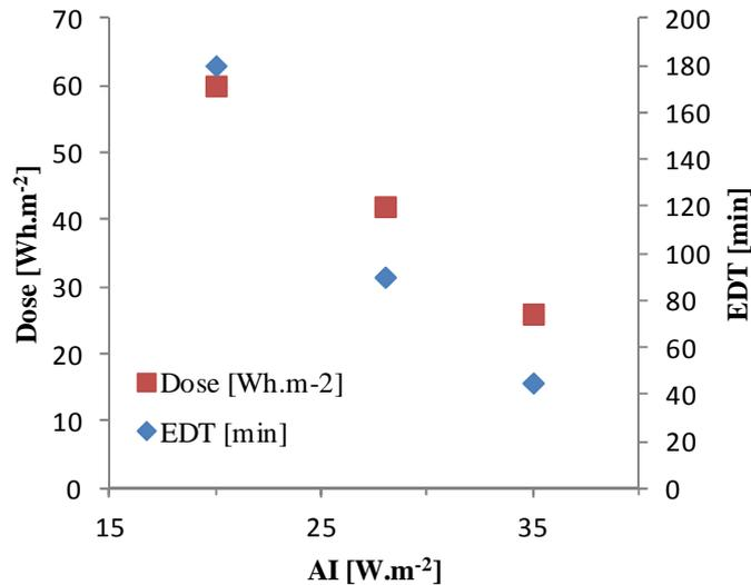
**Figure 3. 4.** Efficient disinfection time (EDT) [min] and dose required for *Salmonella* spp. Total inactivation as a function of average irradiance (AI) [W.m<sup>-2</sup>] available, (■) cumulated total dose [Wh.m<sup>-2</sup>], (◆) EDT (photo-Fenton) [min]: time required for the total inactivation of *salmonella* spp. under photo-Fenton treatment.
