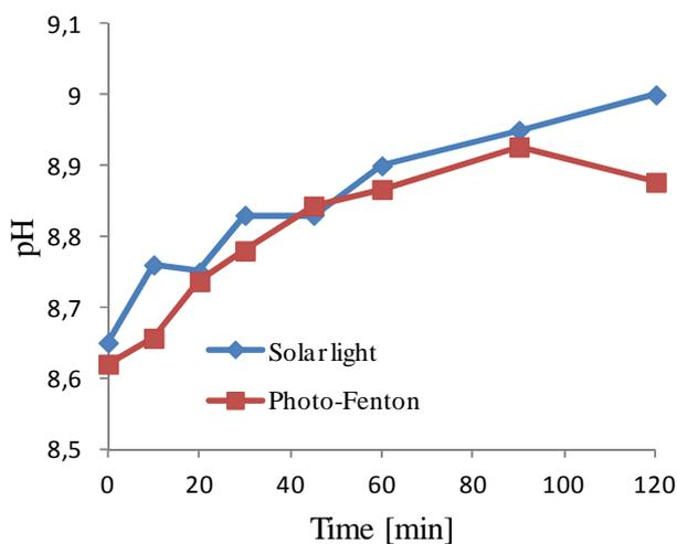
**Figure 4.4:** Evolution of pH during the photo-disinfection treatments: (♦) under solar radiation treatment without  $\text{H}_2\text{O}_2$  addition, (■) under photo-Fenton treatment with 10 mg/L of  $\text{H}_2\text{O}_2$ .
