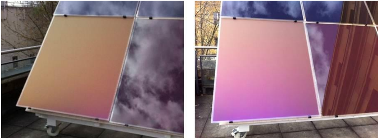
Fig. 4: Orange glass panes laminated on real-size PV modules (1.10 x 1.30 m 2 ) on which strong angular dependency of the color is observed.
