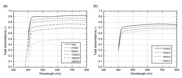
Figure 3: Spectral transmittance of (a) unidirectional specimens at different reinforcement weights and (b) unidirectional and cross-ply specimens
