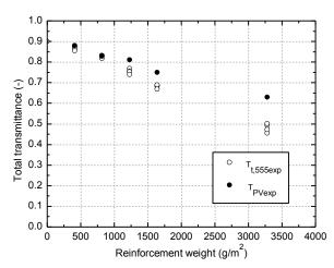
*Figure 4: Transmittance measurements at 555-nm wavelength and from solar radiation flash experiments (UD specimens)*
