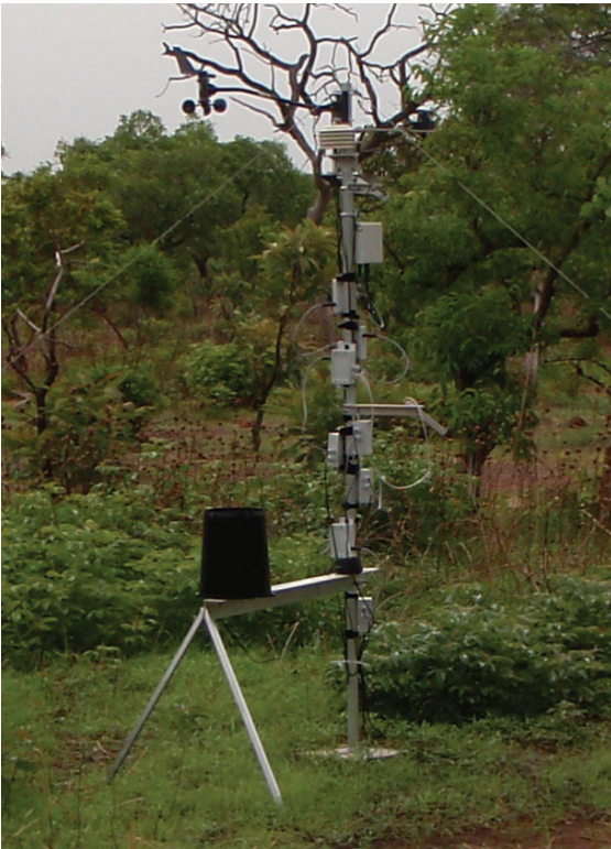
Figure 3-1S. Sensorscope station in the savanna (May 28, 2009). Anemometer, temperature and humidity sensor, surface temperature, radiometer, wires leading to soil moisture sensors, and rain gauge are visible.
