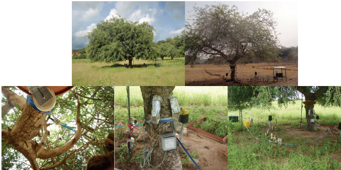
Figure 5-2. Sclerocarya birrea tree in unplanted millet field surrounded by components of wireless sensing network, sap flow sensors, and solar power energy supply.
