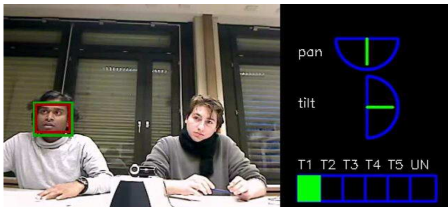
Fig. 4 Tracking, head-pose estimation, and VFOA estimation for an individual in a group interaction in the ELEA AVS corpus. See main text for details.
