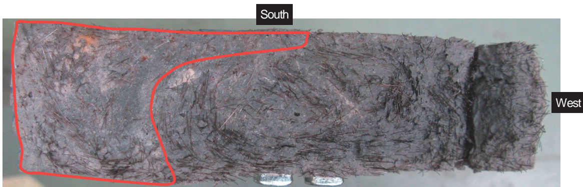
Figure 114 Fatigue fracture surface of S4-4 test specimen (lower half of the fractured specimen)
