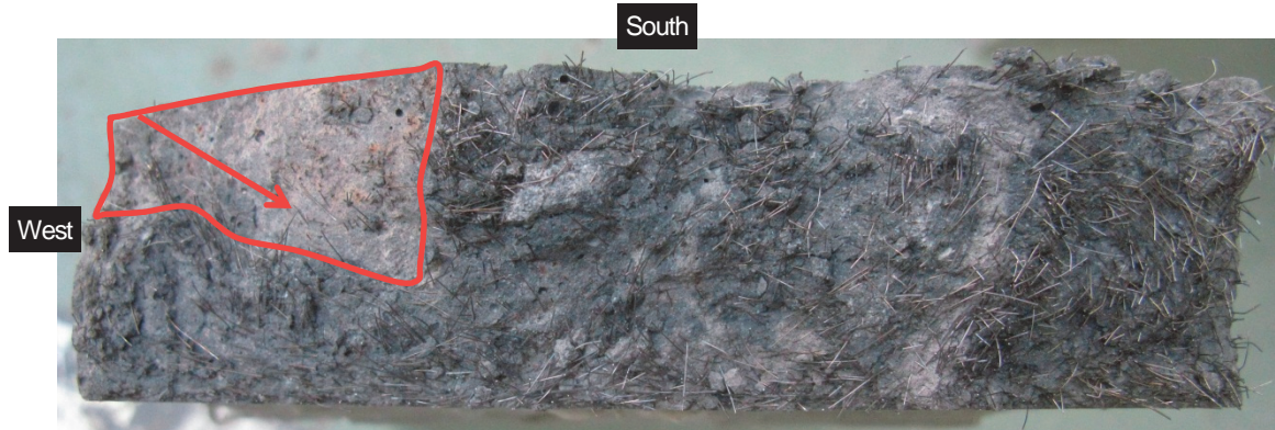
Figure 25 Fatigue fracture surface of S1-2 test specimen (upper half of the fractured specimen)
