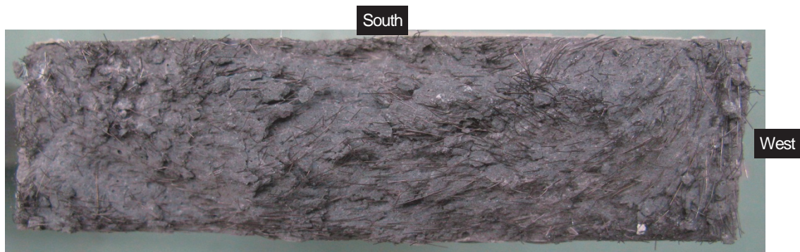
Figure 45 Fatigue fracture surface of S2-1 test specimen (lower half of the fractured specimen)
