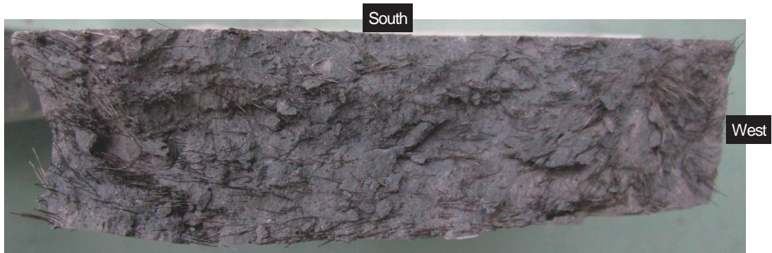
Figure 17 Fatigue fracture surface of Preliminary test 2 specimen (lower half of the fractured specimen)
