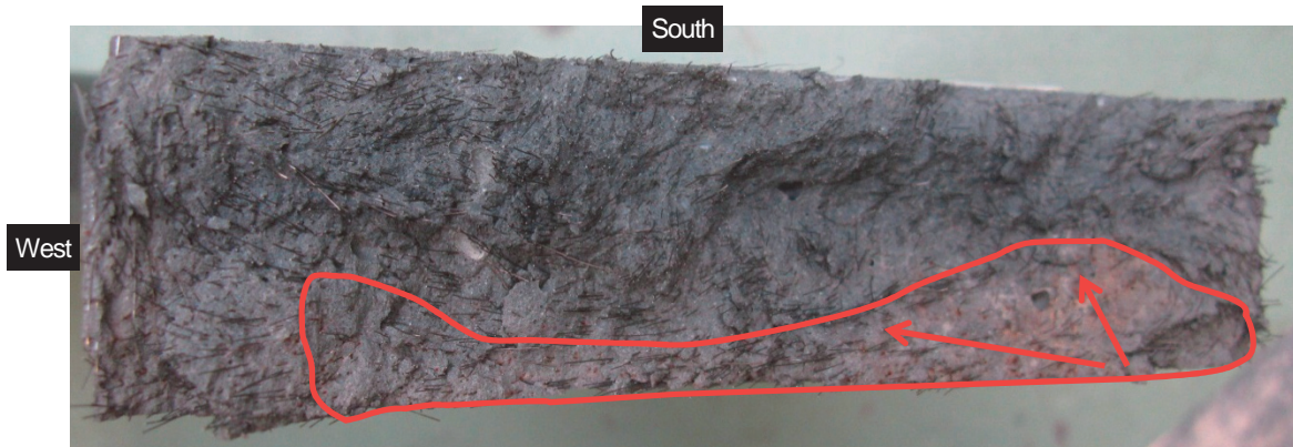
Figure 72 Fatigue fracture surface of S3-2 test specimen (upper half of the fractured specimen)
