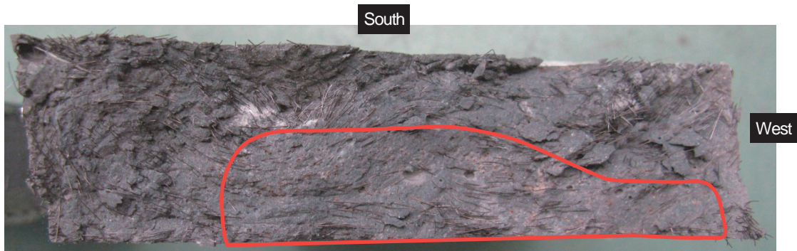
Figure 28 Fatigue fracture surface of S1-3 test specimen (lower half of the fractured specimen)
