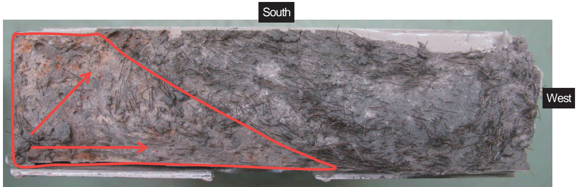
Figure 21 Fatigue fracture surface of S1-1 test specimen (lower half of the fractured specimen)
