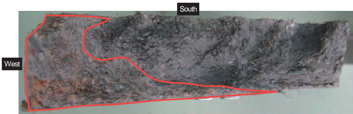
Figure 103 Fatigue fracture surface of S4-1 test specimen (upper half of the fractured specimen)
