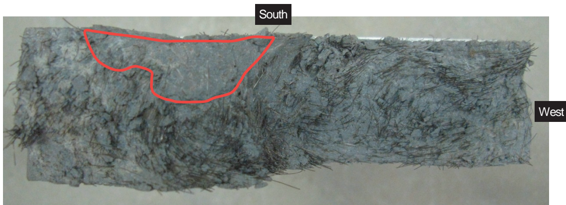
Figure 117 Fatigue fracture surface of S4-5 test specimen (lower half of the fractured specimen)
