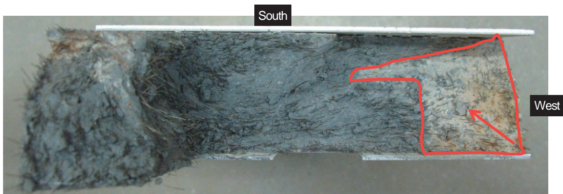
Figure 88 Fatigue fracture surface of S3-6 test specimen (lower half of the fractured specimen)
