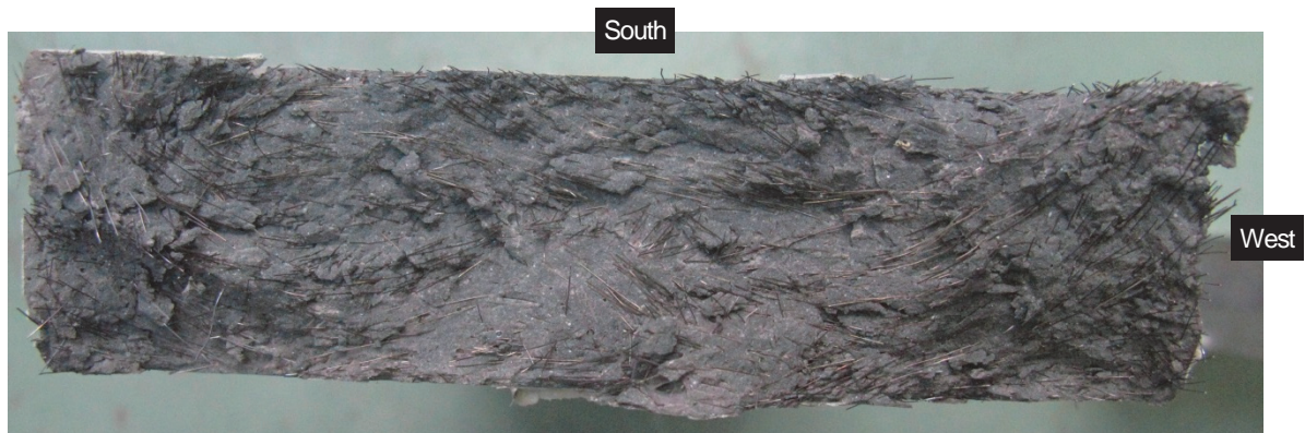
Figure 54 Fatigue fracture surface of S2.5-3 test specimen (lower half of the fractured specimen)
