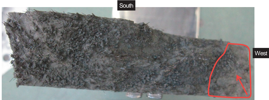
Figure 35 Fatigue fracture surface of S1-5 test specimen (lower half of the fractured specimen)
