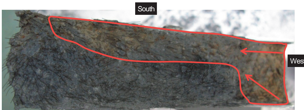
Figure 106 Fatigue fracture surface of S4-2 test specimen (lower half of the fractured specimen)
