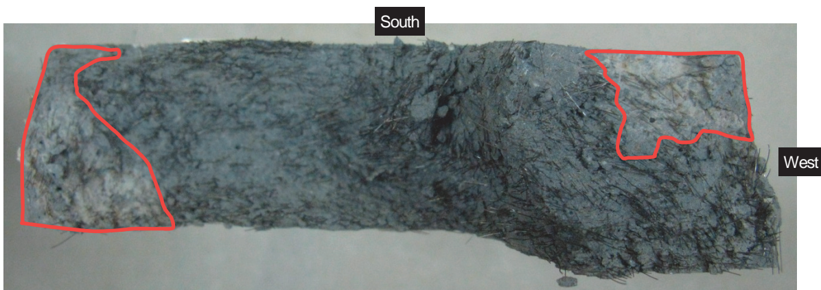
Figure 64 Fatigue fracture surface of S2.5-6 test specimen (lower half of the fractured specimen)
