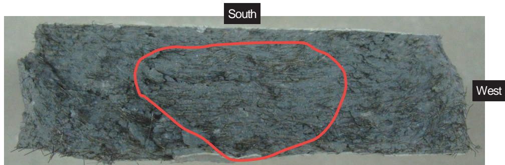
Figure 85 Fatigue fracture surface of S3-5 test specimen (lower half of the fractured specimen)
