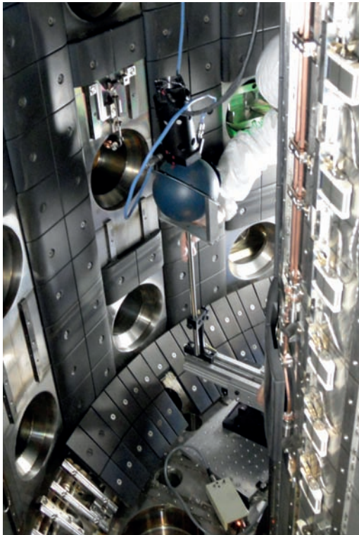
Fig. 3.3.5 Picture showing the absolute calibration sphere placed inside the TCV vessel during the TCV 2012 vacuum opening.
