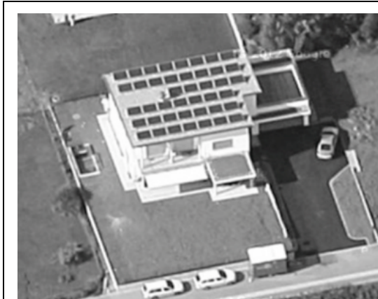
Figure 1: Test system on a flat roof with 36 m 2 collector area. Source: Google Earth
