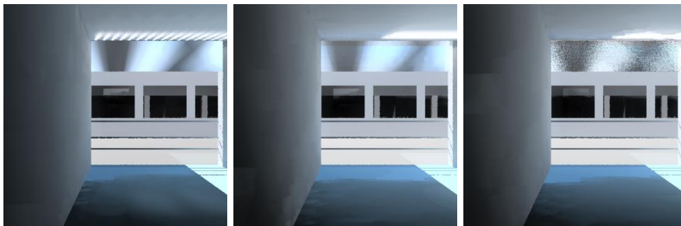
Figure 1. Visualization of the office room using mkillum with the full-size window (left); the visualization using mkillum with the subdivided window (center) and the visualization obtained with the bsdf procedure (right).
