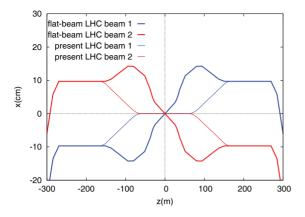
Figure 3: LHC reference orbits in the straight section for the new flat-beam optics, compared with the present LHC.
