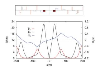
Figure 2: LHC flat-beam IR optics for Beam 1. Bending magnets are shown in blue, quadrupoles in red and sex-tupoles in black. The DHQ is shown in black and red stripes.
