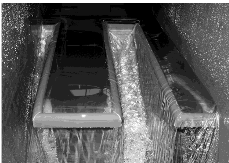
Figure 3. Flow features on sectional PKW model ( T_s = 2R = 0.02 m, cylindrical crest) under a small head (Leite Ribeiro et al. 2012)
