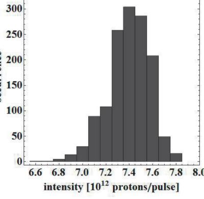
The spot size at the target is determined by the beam optics, validated during the commissioning tests, while the beam position and intensity are quite stable from pulse-to-pulse.
