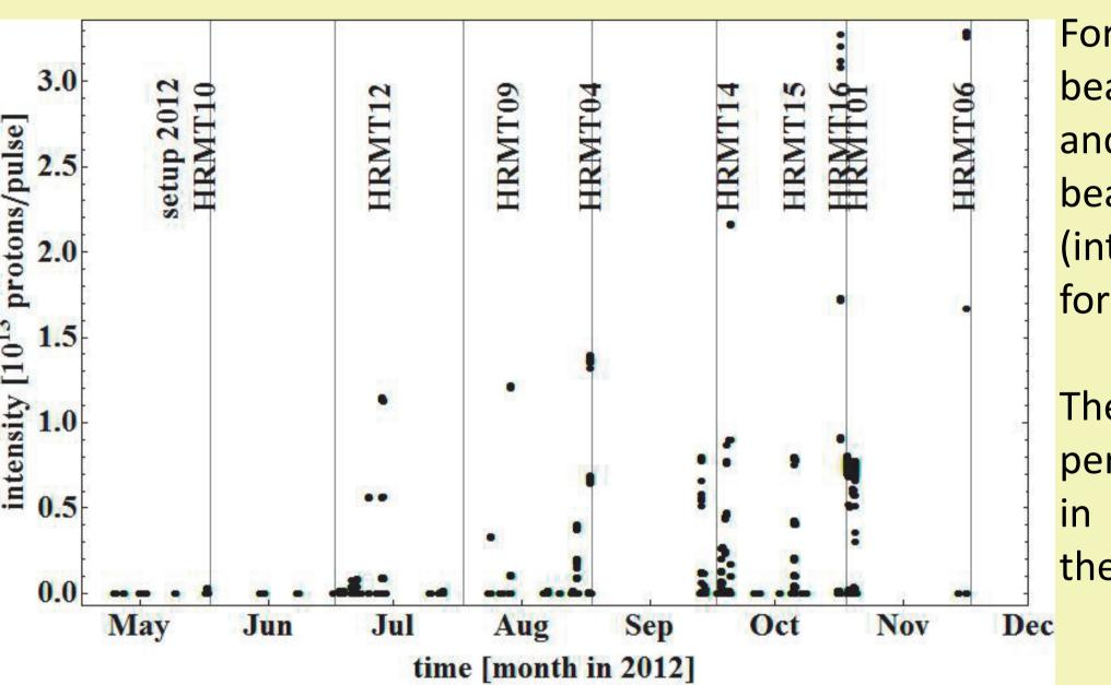
For the HiRadMat experiments, the interesting beam parameters are the intensity, spot-size and repetition rate for the beam pulses. The beam intensity is measured for each pulse (integral) and per bunch using current transformers in the line.
