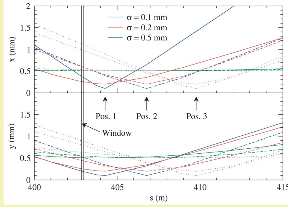
The beam size and the focal position are fully adjustable along the experimental target positions.
