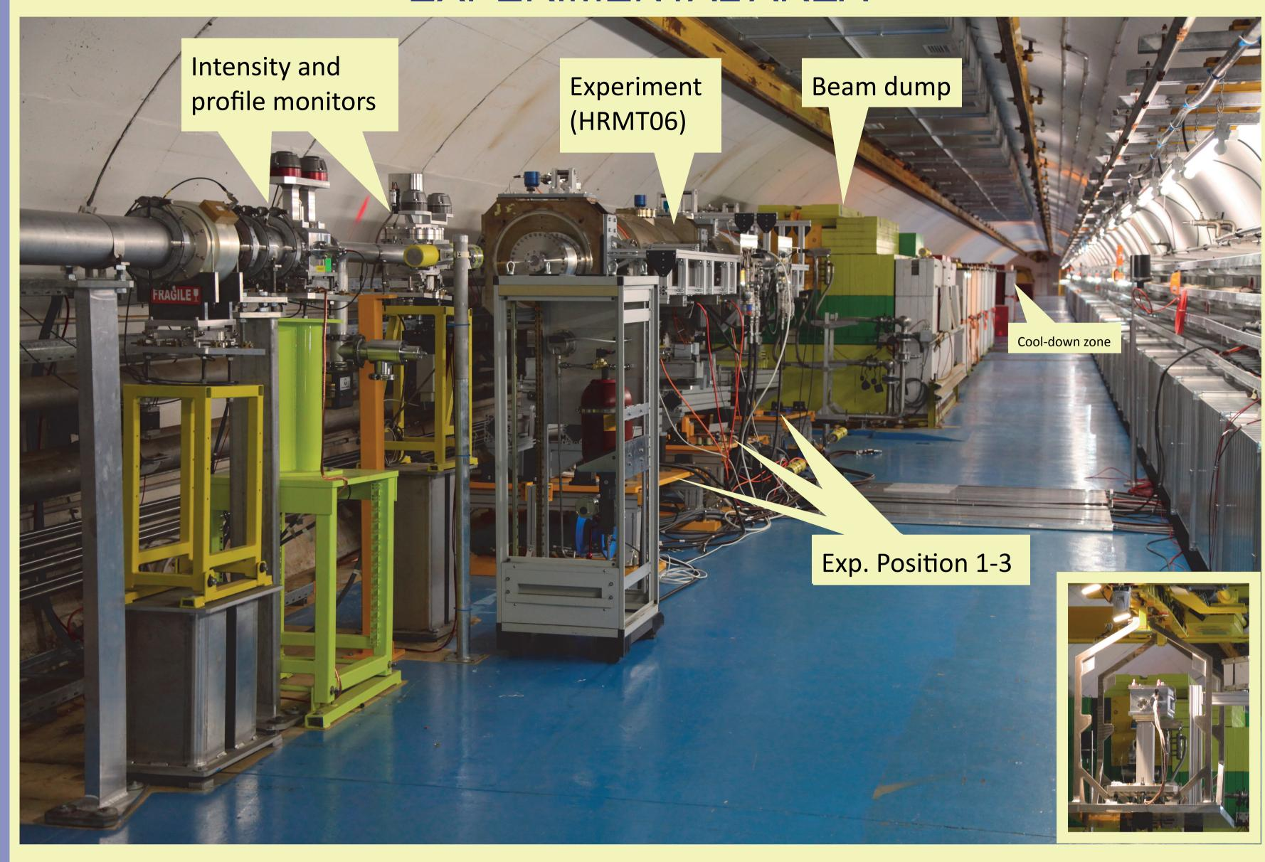
The HiRadMat experimental area is located at the TNC tunnel (ex. WANF facility target & secondary beam tunnel) in the SPS-BA7 area. The facility offers the possibility of three test stands receiving beam at the same time. Installation of the test material is done remotely using specially designed platforms.
