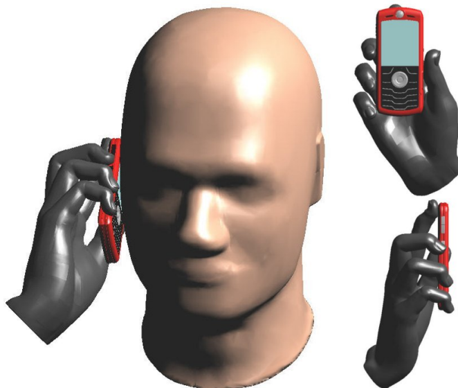
Figure 6.6: The SAM head phantom cheek placement and a CTIA-compliant hand phantom grip for the investigated mobile phone.
