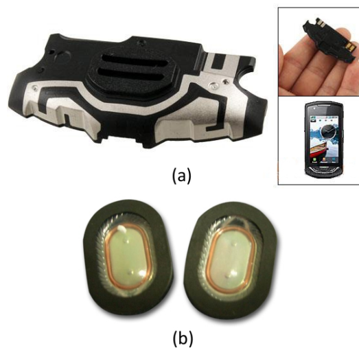
Figure 1.3: (a) A typical antenna-speaker assembly module and (b) miniature speakers to be integrated.
