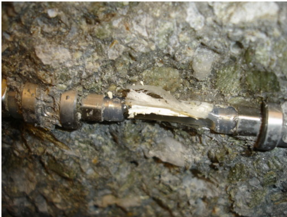
Figure 2.11: Buckling failure of a fibre-optic sensor cast in a concrete sample exposed to 5 MPa water pressure.
