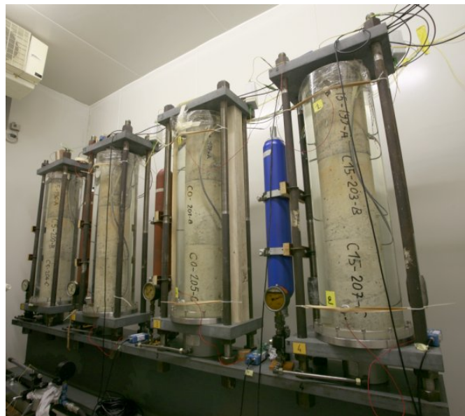
Figure 2.2: Experimental setup for study of ASR under uni-axial load and immersion in alkaline solution from [12].
