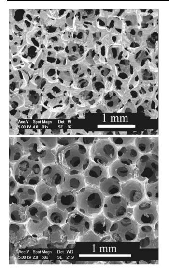
Fig. 2 Replicated foam with 400  $\mu$ m pore of irregular polygonal shape (*top*) and spherical shape (*bottom*)
