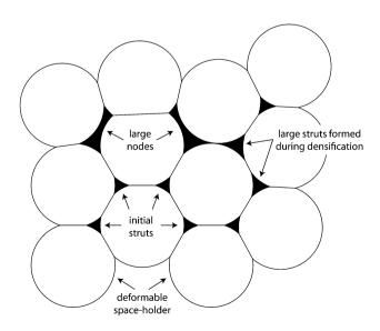
Fig. 1 2D schematic of the space between close-packed and partly densified spheres
